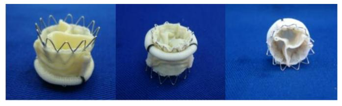
Fig. 3 - Image showing the structure composed by the overlapping of a conventional prosthesis (27 mm) and a transcatheter prosthesis (26 mm).
